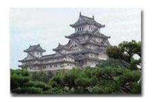
Although elegant and refined in appearance, Japanese castles were used as military installments. The wood used in their construction allowed these castles to withstand Japan's many earthquakes, but made them susceptible to fire at the same time.
